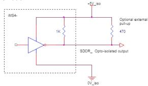
Diagram shown with optional external pull-up resistor to improve the rising edge. Min value 330ohm
