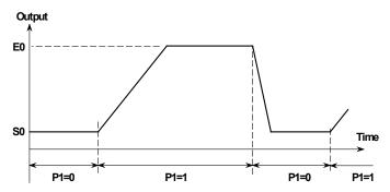
Both plots show a ramp on output J2, controlled using input P1
